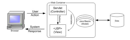
Figure 3-5.The Struts framework uses a Java servlet to handle the controller responsibilities
