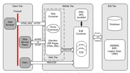
Figure 2-2. The Struts framework is used within the Web Tier
