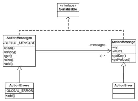
Figure 7-5. ActionErrors are Specialized ActionMessages
