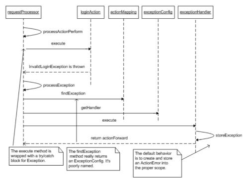
Figure 10-3. A Sequence Diagram for Struts Exception Handling
