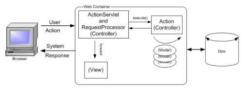
Figure 3-6. The execute() method of the Action class is called by the primary controller
