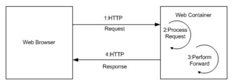
Figure 2-8. During a forward, the request is sent to a secondary resource on the server without notifying the client
