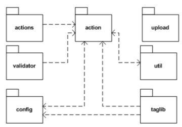
Figure 3-4. The Struts framework consists of 7 top-level packages
