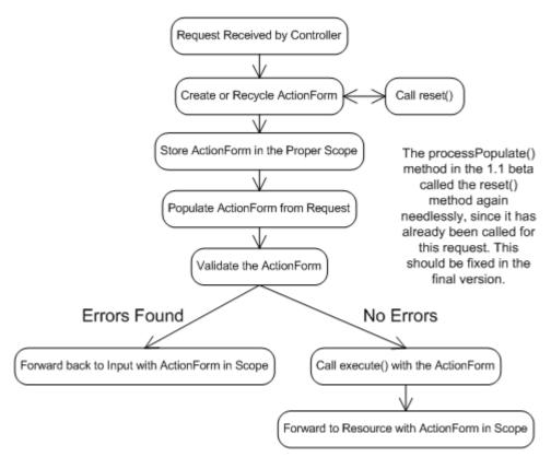
Figure 7-4. The Life Cycle of an ActionForm
