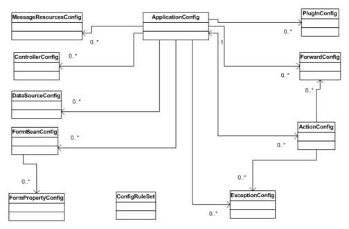
Figure 4-4. The class diagram of the org.apache.struts.config package
