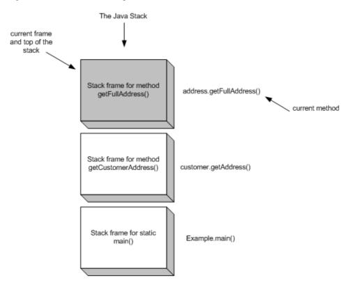
Figure 10-2. An example of a Java method invocation stack (call stack)
